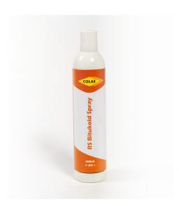
**RS Bitukold** is a rapid setting, cold applied thixotropic bitumen emulsion designed for sealing vertical joints. The cationic formulation of **RS Bitukold** ensures a rapid set even in cold, damp conditions, with an initial cure taking place within 15 minutes. **RS Bitukold** is mainly used for the protection of new joints in freshly laid asphalt or macadam.
