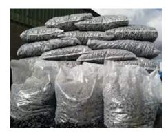
Pre-Coated Chippings are rolled into hot rolled asphalt to form part of the surface. They are resistant to polishing and can be used as part of the laying process to achieve the desired skid resistance which is 65psv in all types of roads from motorways to housing estates. Pre-Coated Chippings let you reinstate even the smallest of hot rolled asphalt patches without having to buy the chippings by the tonne.
