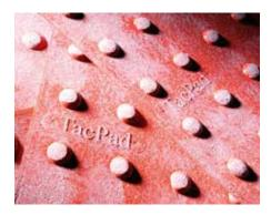
**Tac-Pads** are a two part system and are installed to alert blind and partially sighted people to proceed with caution. **Tac-Pads** are easy to apply, can be trafficked immediately and are available in red, buff or grey. **Tac-Pads** are non-toxic, contain no lead or chromate pigments and are skid resistant to >55 SRV.
